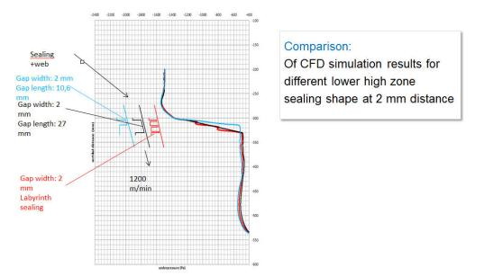
Figure 06. CFD simulation results for the three different sealing (labyrinth sealing with 3 slices, single sealing 10 mm and single sealing 27 mm width)
