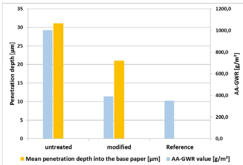
*Figure 3:* Penetration depth of lignosulfonates into base paper (measured according to Hofer et al. (2015)) and AA-GWR water retention of coatings containing lignosulfonates from spent liquor compared to the reference (untreated... lignosulfonate from spent liquor, no treatment; modified... enzymatically polymerized lignosulfonate from spent liquor)
