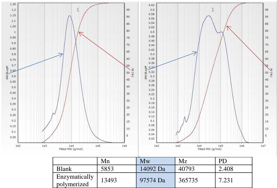
Figure 4: Molecular weight distribution (SEC) of enzymatically polymerized lignosulfonate (ultrafiltrated  $2\mu\text{m} > x > 150\text{kDa}$ ) with 30% TDS (right) compared to blank (untreated ultrafiltrated lignosulfonate) at 30% TDS (left, no enzyme treatment) and their average molecular weights (table below figures)
