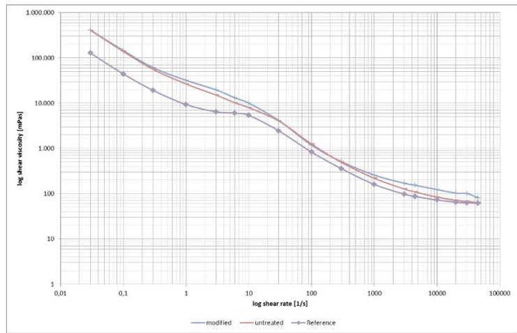
Figure 5: Rheological behavior of untreated (ultrafiltrated, no enzyme treatment) and modified (ultrafiltrated, enzymatically polymerized) lignosulfonate containing coatings in comparison to reference coating
