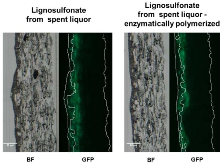
Figure 1: Penetration of lignosulfonates from spent liquor into the base paper. Brighfield (BF) and green fluorescent (GFP) images of blank (untreated lignosulfonate from spent liquor) (left) compared to BF and GFP image of enzymatically polymerized lignosulfonate from spent liquor (right).
