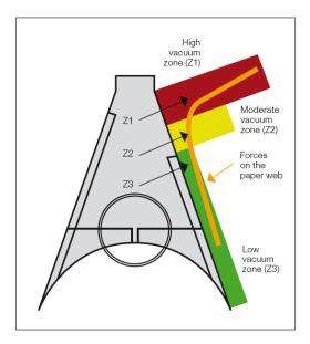
Figure 3: Andritz solution: PrimeRun Evo, three different zones, depending on the vacuum needed, neutralize the forces and stabilize the web.
