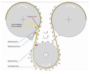
Figure 1: Single-tier drying sections – forces that affect the web runnability
