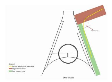
Figure 2: The runnability concept of today (two zones controlling web stabilization: 1) high underpressure zone and 2 low underpressure zone)
