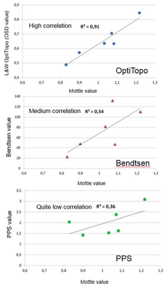
Figure 24 - Case study where OptiTopo proved to be better compared to air leak methods at predicting mottle value [10].
