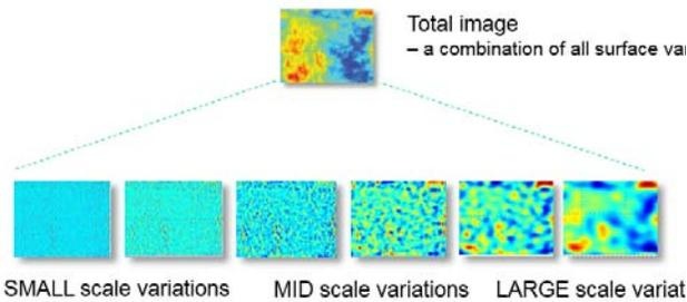
Figure 15- Result after 2 dimensional FFT analysis. Variations in topography are divided into small scale, mid-scale and large scale variations
