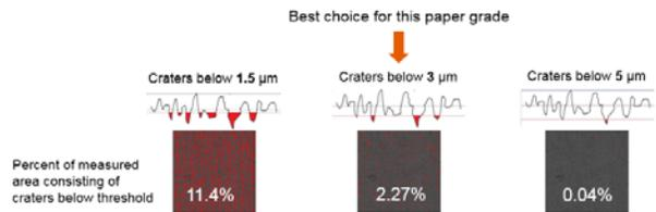
Figure 17 - Crater measurement on the same sample with three different thresholds
