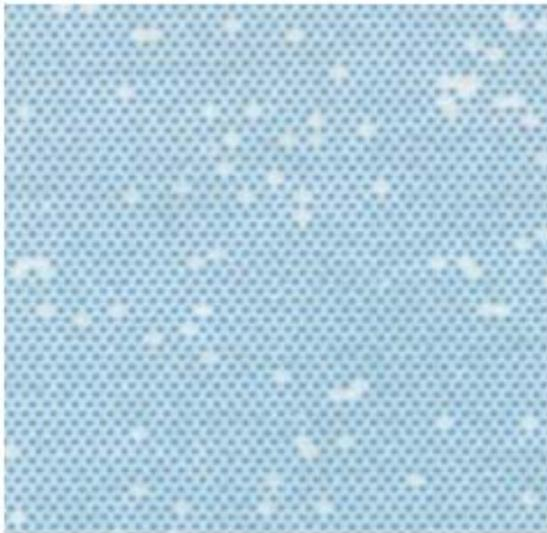
Figure 9 – Example of Missing Dots defects
