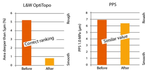
Figure 23 - PPS could not identify the improved surface whereas OptiTopo clearly measured a difference before and after [10]
