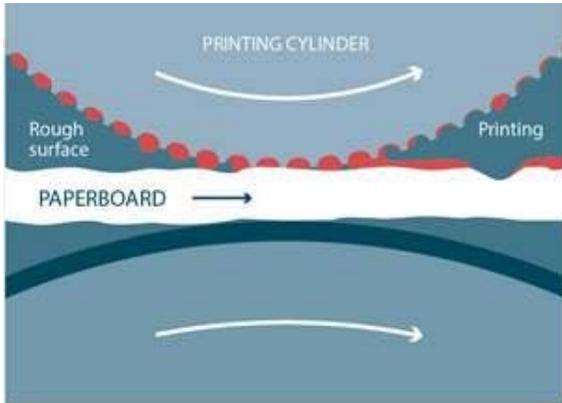
Figure 8 - Crater causing a missing dot
