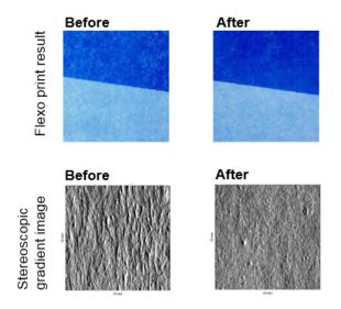
Figure 22 - Example of reduced mottling and UCA after machine rebuild. [10].
