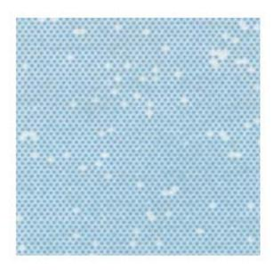
Figure 9 – Example of Missing Dots defects
