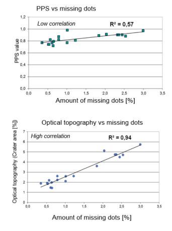
Figure 21 - Comparison between PPS and optical topography crater measurement versus missing dots [10]
