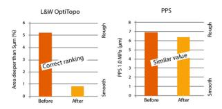
Figure 23 - PPS could not identify the improved surface wheras OptiTopo clearly measured a difference before and after [10]
