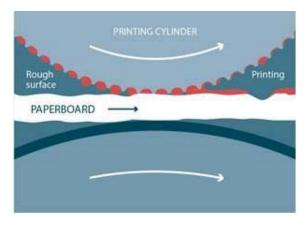
Figure 8 - Crater causing a missing dot
