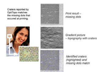
Figure 19 - Missing dots in test print matches the craters identified by OptiTopo
