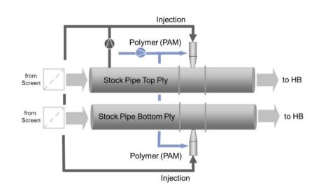
Stock suspension used for injection Chemical at high concentration
