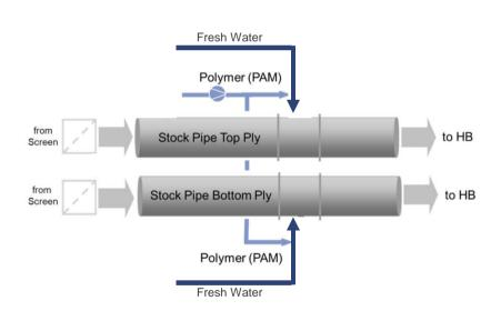
Fresh water used for injection Chemical at low concentration
