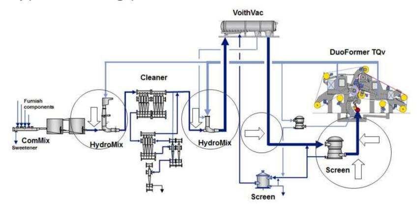
All dosing position along the process line in thin- and thick-stock.
