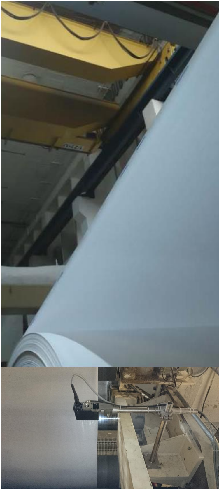
| Figure 6: A kilometer code marked at the edge of the jumbo roll at unwinding (top) and the code reader
