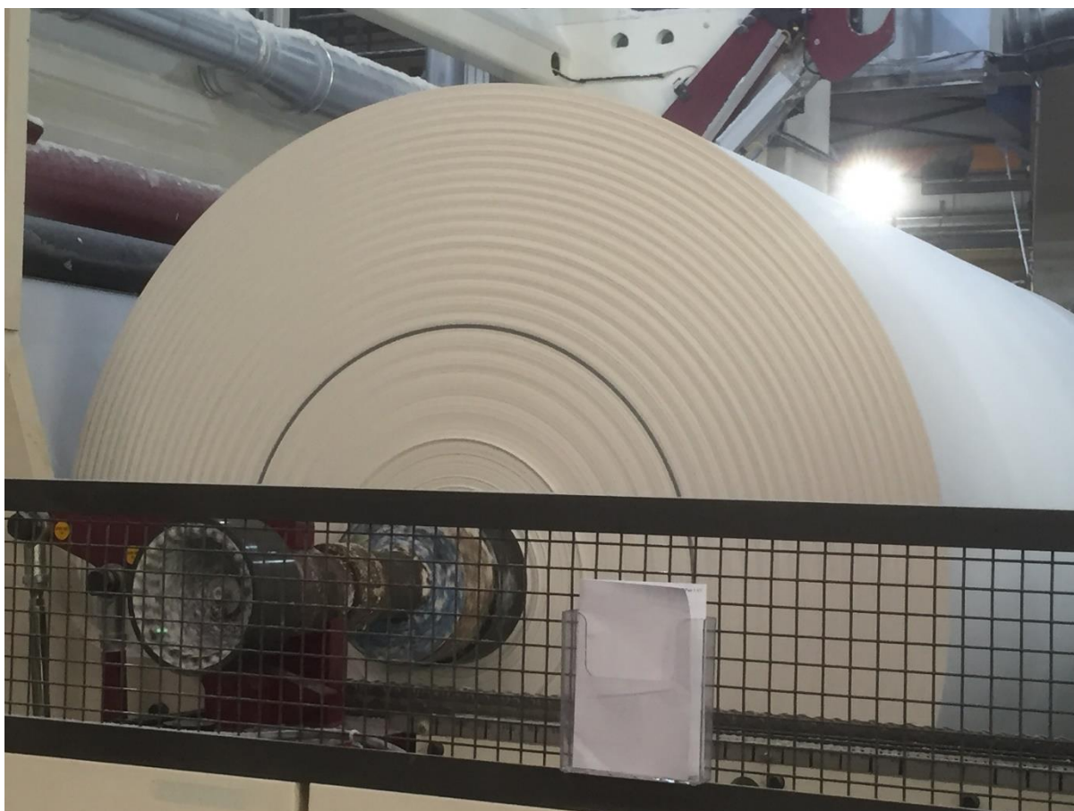
Figure 7 : A defect color marked at the end of the jumbo roll
