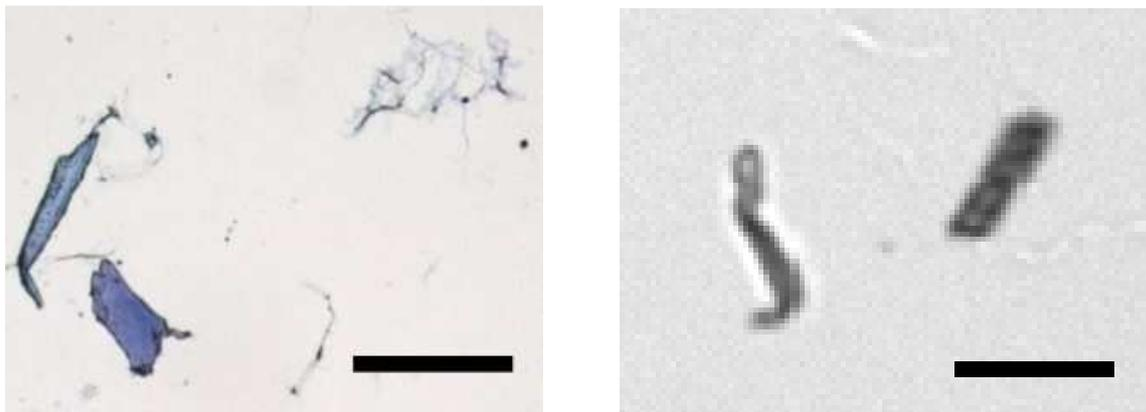
Figure 1: Images (microscope: left; fibertester: right) of F4 fines; black bar: 100 $\mu$ m
