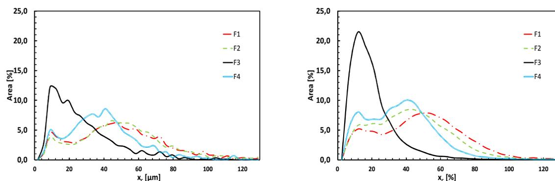
Figure 2: Particle size distribution; microscope (left diagram): only flake like material is measured; automated analyser: (right diagram): all material (flakes + fibrils) is measured
