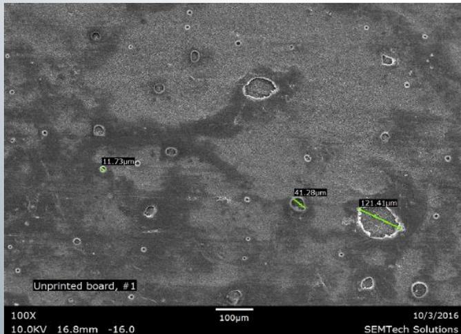
Low VE causes the air entrainment by literally pulling the air underneath the coating
