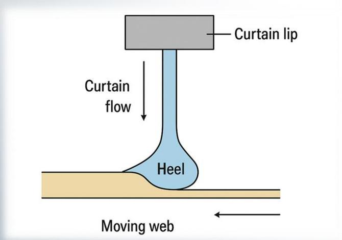
Not proper extensional viscosity (usually too low) causes a heel formation
