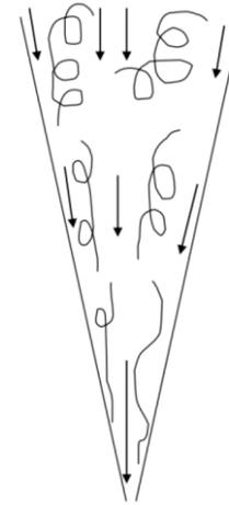
$$\text{Extensibility} = \frac{\text{Polymer chain length } (L_{CH})}{\text{Coil radius } (R_G)}$$
