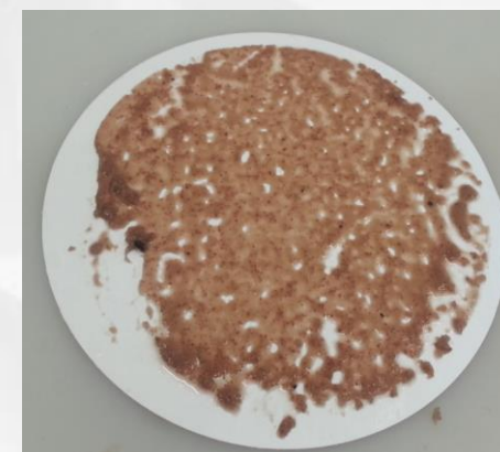
peeled corn cobs – attempt to form laboratory sheet
