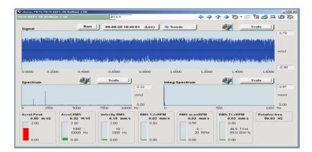
When a vibration alarm is acknowledged and activated by a mouse click on the combined process display a pop-up window reveals the details of the vibration patterns in the process element. From here, a precise diagnosis can be made.
