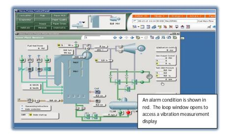
A machinery condition alarm generates a visible alert on a typical DCS process display. When this alarm is activated by a mouse click a detailed vibration analysis window opens as shown below.
