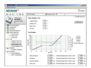
Remotely-initiated tests like this, as well as the continuing online diagnostics, determine the health of a valve and when to make necessary repairs.
