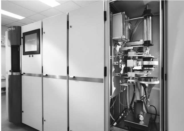
L&W Pulp Tester – for automatic pulp testing according to industry standards..
