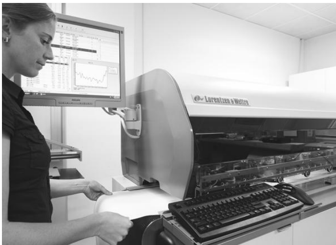
A paper sample is fed into the L&W Autoline system and measurements start automatically.
