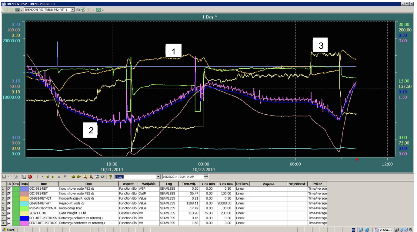
Fig 7: Trend of polymer closed loop control
