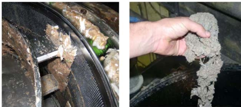
Figure 5. Stringy contaminants can hang up on the rotor foils and form into larger clumps which have the potential to jam between the cylinder and rotor.
