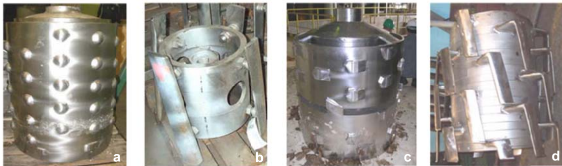
Figure 1. Some different rotor designs have come into use since pressure screens were introduced in the 1960s including: a) the “bump-type” rotor from the 1960s, b) the “stud-and-nut” foil rotor (1970s), c) a “modified bump” rotor (1990s), and d) a cantilever foil rotor (2000’s).
