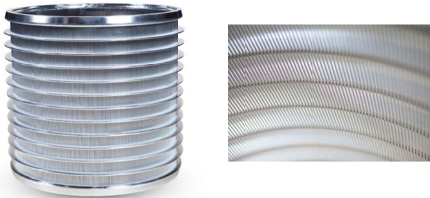
Figure 8. The AFT MacroFlow2 wedgewire cylinder is shown on the left, with a series of support rings holding the wedge wires that define the slots. A close-up of the interior (feed-side) of the cylinder is at the right.
