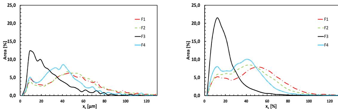
Figure 2: Particle size distribution; microscope (left diagram): only flake like material is measured; automated analyser: (right diagram): all material (flakes + fibrils) is measured
