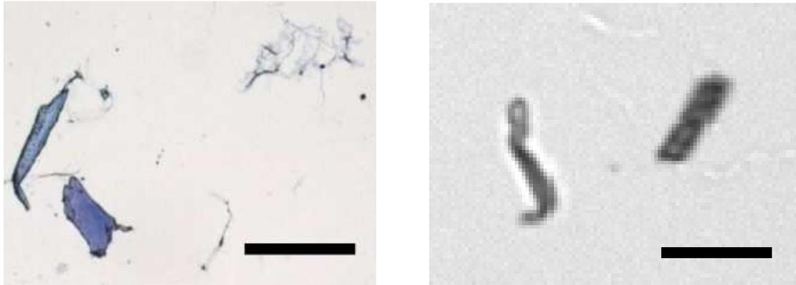
Figure 1: Images (microscope: left; fibertester: right) of F4 fines; black bar: 100 $\mu$ m
