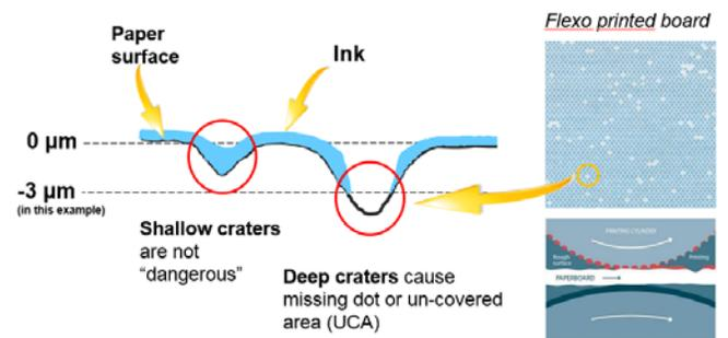
Figure 18- Craters below a certain depth can cause missing dots
