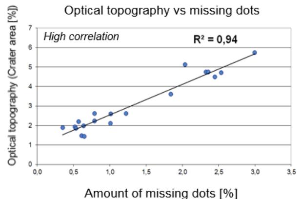
Figure 21 - Comparison between PPS and optical topography crater measurement versus missing dots [10]
