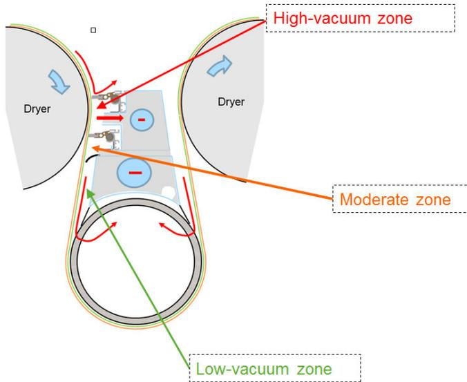
Figure 02: Working principle of three zone PrimeRun Evo model
