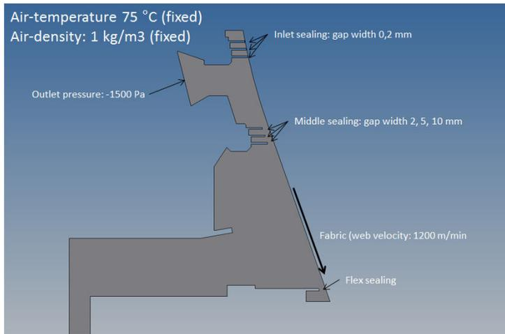
Figure 05: Boundary conditions for the three zone model
