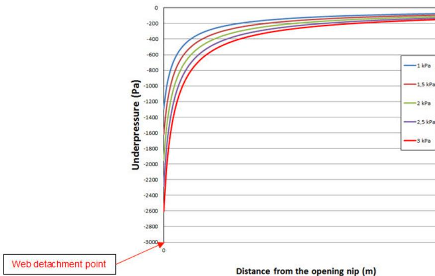
Figure 03: Underpressure distribution as a function of distance from the opening nip and box underpressure (Juha Leimu, The paper machine cylinder opening nip, LAP LAMBERT Academic Publishing)
