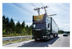
This new system, which works through overhead lines on the right lane of the highway, will be compatible with HDVs utilising different drive technologies, including purely electrical and hybrid vehicles with diesel, bio-diesel, gas and batteries. Thereby, the vehicles will be able to recharge their batteries while driving under the overhead lines.
