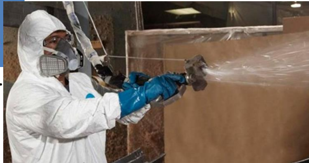
The lay-up of the reinforcing fibres / resin mixture with the chopper gun.
