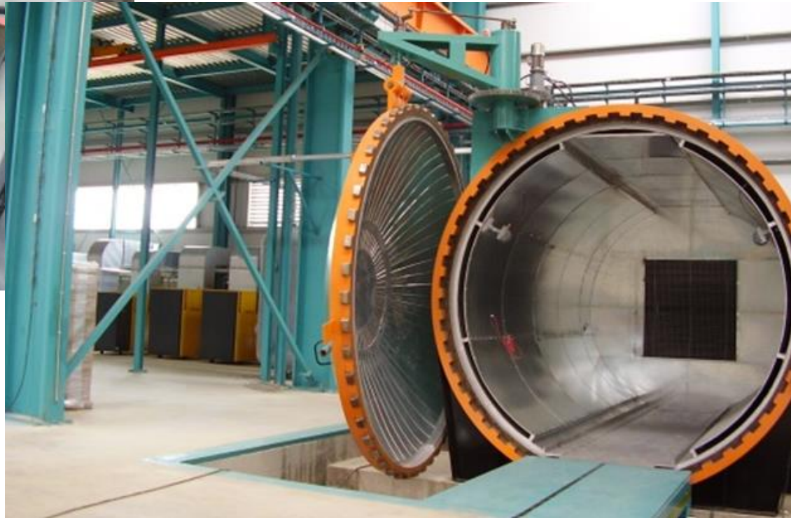
An example of autoclave moulding setup.
