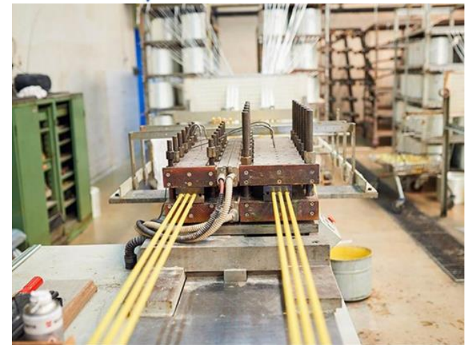
The photo of the finished GFRP rods at the end of the poltrusion process.
