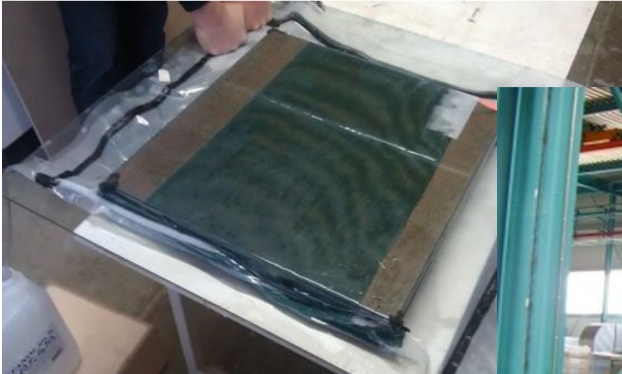
Preparation of simple FRP plate by vacuum bag moulding.
